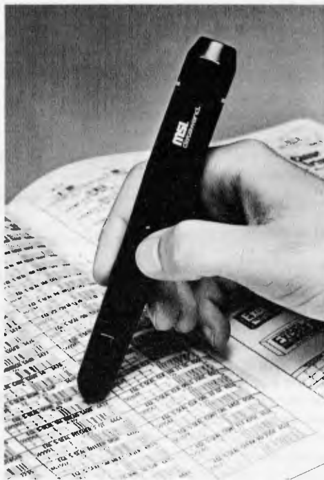
Datawand portable scanner can collect, decode, delete and transmit data.
